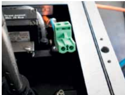
FIGURE 4 Replace the old 2-pin fieldbus connector with new 3-pin connector
