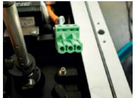
FIGURE 4 Replace the old 2-pin fieldbus connector with new 3-pin connector
