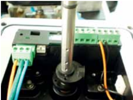
FIGURE 5 New electronic module installed with I/O connectors on
