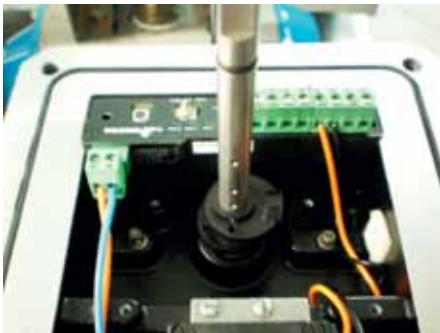
FIGURE 5 New electronic module installed with I/O connectors on
