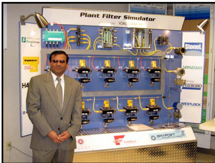
Vijaykumar Soni in front of the Fieldbus Foundation's FFB display demo with 10 Westlock 7344 Fieldbus Control Monitors. The Foundation used this display at the ISA Expo 2005 Fieldbus booth.
